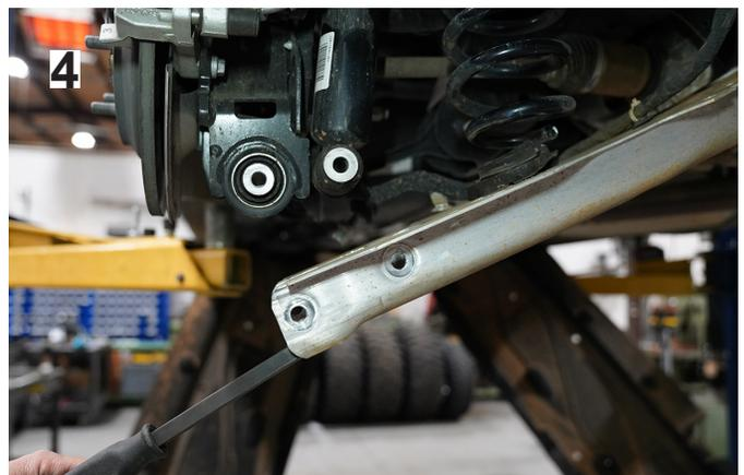
10. [Illustration 6] Remove the coil spring isolator from the lower control arm and drill the hole out to 6mm or 0.25".
