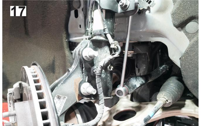
26. Reattach the tie rod end to the knuckle. [15mm]
