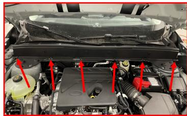
Lift up the cowl and remove the two 10mm bolts retaining the strut cover.
