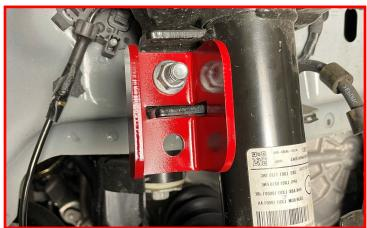
Mount the End Link to the End Link Drop Bracket using the supplied hardware.
