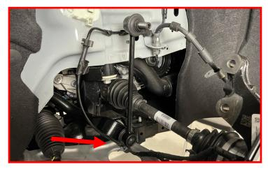
Using a sanding disk, grind down the inboard edge on the bottom of the strut so it's flush with the strut body.
