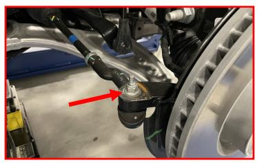
Strike the side of the steer arm to remove the tie rod from the knuckle.
