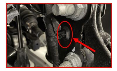
Remove the brake line bracket with an 8mm wrench.
