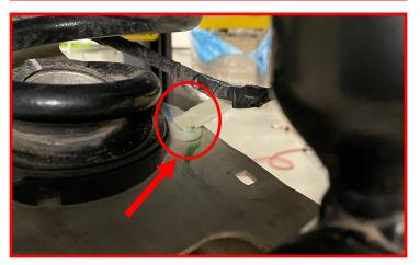
Carefully remove the spring from the lower spring isolator. A pry bar may be needed. Let the spring hang.
