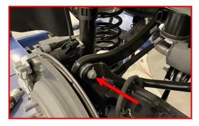
Loosen, but **DO NOT REMOVE**, the rear trailing arm 15mm bolt.
