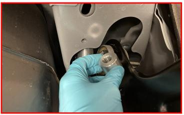
Bolt in the trailing arm using the supplied M14-2.0x60mm bolts, M14 flat washer, and lock washer.
