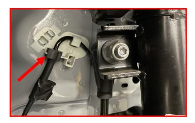
Remove the ABS wire from the strut
