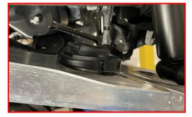
To access the trailing arm bolts, lower driver side the sound dampening liner by removing the three 10mm nuts and two screws.
