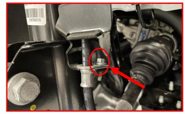
Remove the 15mm tie rod nut.
