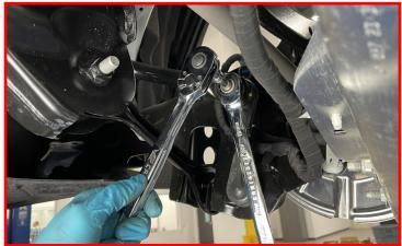
Loosen, but **DO NOT REMOVE**, the upper control arm 15mm bolt.
