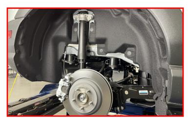
Remove the end link nut using an 18mm wrench and a T40 Torx.
