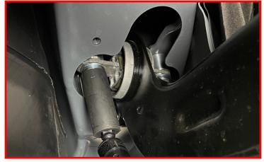
Torque the rear trailing arm hardware to 80 ft-lb.
