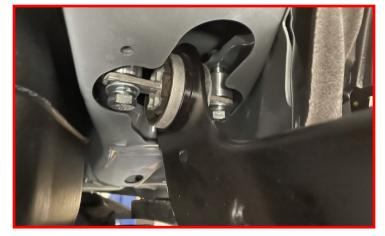
Install the Rear Strut Spacer and factory spring isolator.
